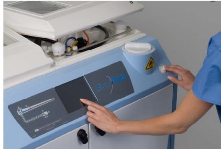
Figure 46. Simultaneously press BOTH Buttons To Close The Lid.
