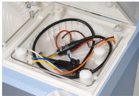
Figure 45. Make sure no tubing sets protrude above the rail.
