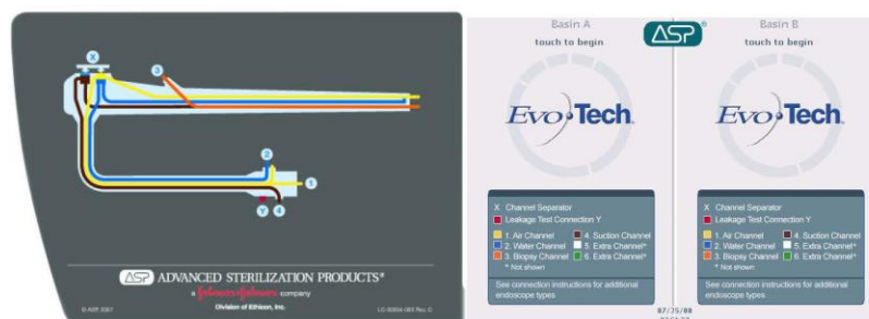
Figure 41. This figure shows both the Tubing Set Diagram on the front panel and the color-coded channel information shown on the display screen.
