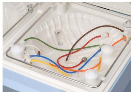
Figure 42. Tubing set attached to color-coded and numbered connections. Shown without a scope for clarity.
