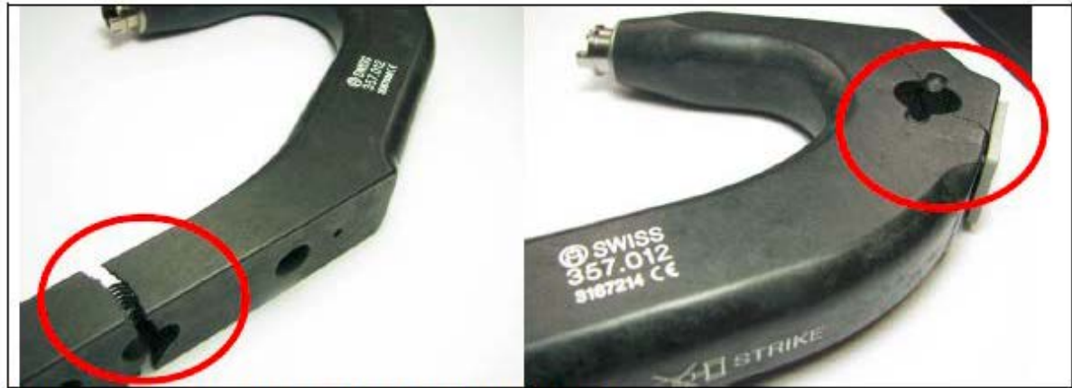
Pictures: Example of broken Insertion Handles 357.012
