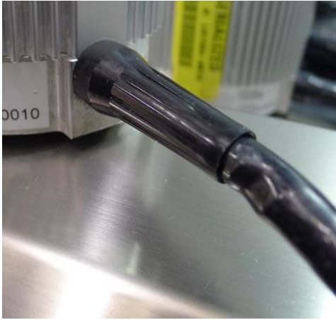
Figure 5: Cable Damage at the Motor Bend Relief
