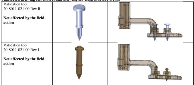
As indicated in the pictures above, drawing revision M to P of the Drive Pins has an X cross section instead of circular. Also, the Drive Pin head has a recess in the enlarged head. Only iASSIST Validation Tools with drawing revision M to P Drive Pins, in the red box above, are affected by this field removal.
