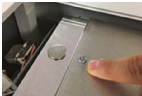
Figure 5: Locating the Back Reflector Screw Nut
