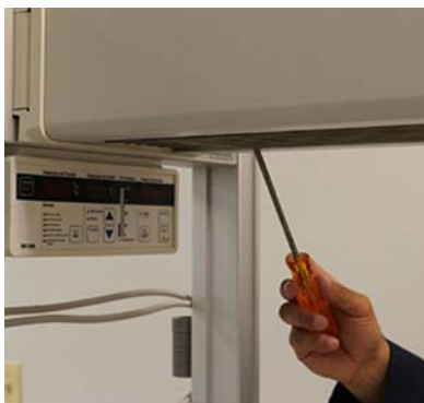
Figure 8: Engaging the Back Reflector Screw
