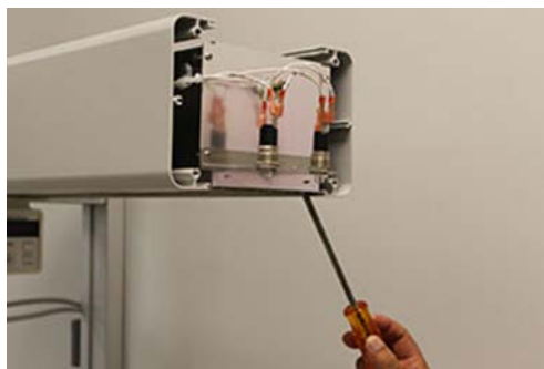
Figure 6: Engaging the Front Reflector Screw
