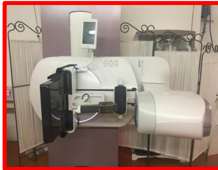
Figure #3 – Do Not Use Gantry Rotation for Biopsy Procedure: Senographe Pristina gantry rotated at 90° position.
