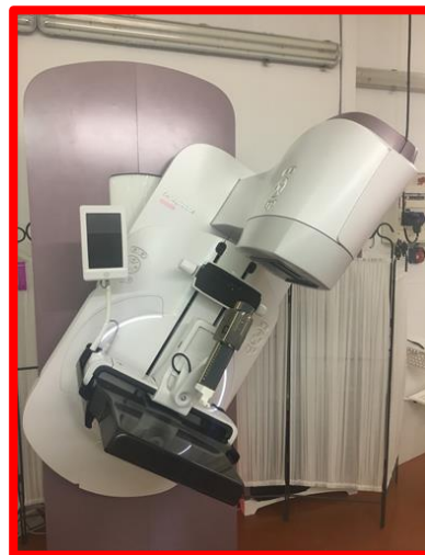
Figure #4 – Do Not Use Gantry Rotation for Biopsy Procedure: Senographe Pristina gantry at ANY rotation different from 0°.
