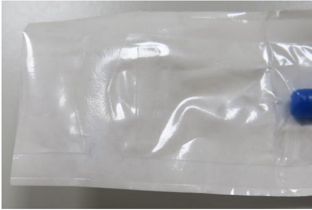
Example of chevron seal - potentially not present
