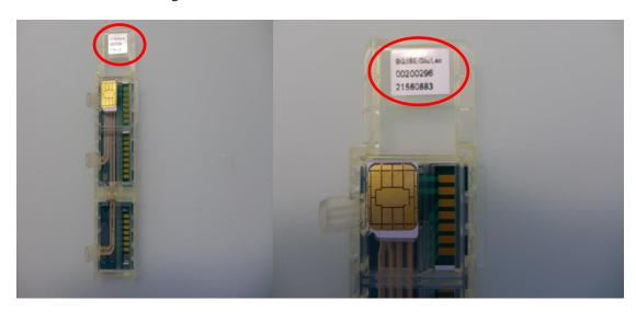
The lot number of an installed Sensor Cartridge can be checked in **cobas b** 123 system software under "Instrument > Consumable Status > Sensor Cartridge".
