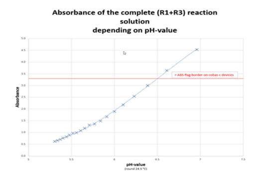
Absorbance of the complete (R1+R3) reaction solution depending on pH-value
