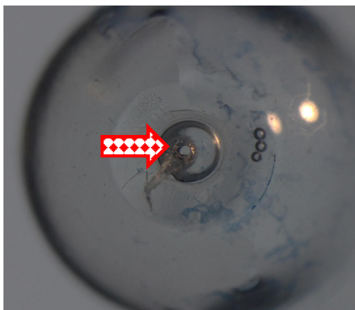
Figure 3: Example of a damaged AssayCup with the small hole at the bottom, which can only be seen with magnifying glasses. The small hole is marked by the red arrow. Blue colored water and the three water droplets next to the small hole are the result from previous investigations.
