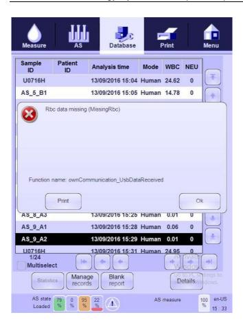
If manually operating the system, the message must be cleared to continue. If running samples with the autoloader, the instrument will continue to process samples when the dialog box appears.
