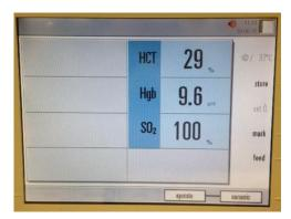
**Connected:** The CDI System 500 monitor displays a value or an indicator of "High" or "Low" in the HCT, Hgb, and SO<sub>2</sub> fields. There is no error message for the "H/S DISCONNECT AT CUVETTE" displayed in the upper left corner of the monitor.
