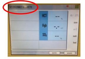
**Not Connected:** The "H/S DISCONNECT AT CUVETTE" error message displays in the upper left corner of the monitor display. This error message indicates that the CDI H/S Cuvette <u>has</u> <u>not</u> established connection to the CDI H/S Probe.
