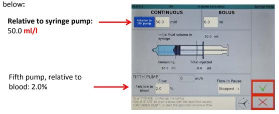
2. If you press on the **blue button**, the constant flow of the syringe pump is activated and
