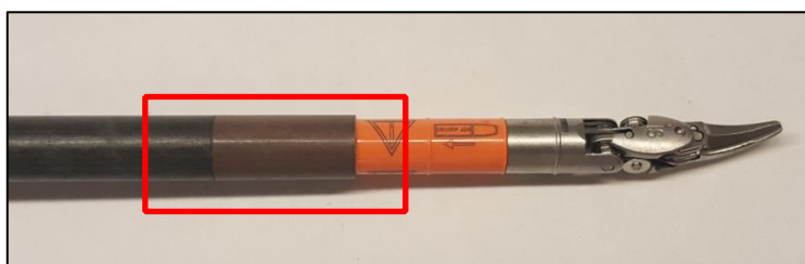
Figure 1. da Vinci S/Si EndoWrist MCS with proximal edge of extension tube highlighted.
