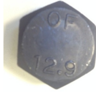
Fig. 1 Faulty bolt with 'OF' on face of bolt.
