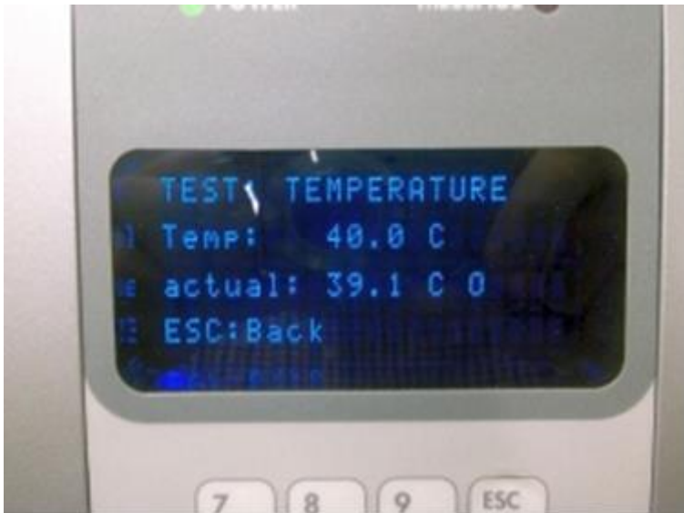
Figure 1. EZ1 Advanced XL display following a successful temperature check. Note specifically the "O" after the "actual" temperature
