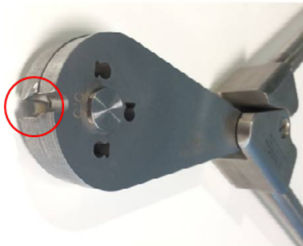
Figure 1. MESA Rail Cutter with damaged blade (see circled area)
