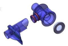
We have detected premature hardening of the silicone membrane, depending on the product used, during the immersion disinfection phase. The rigidity of this membrane may have a negative impact on the quality of ventilation when the PEEP (Positive End-Expiratory Pressure) is set at 0 cmH20 or is virtually zero. It may cause a leak at the expiratory valve, which does not allow the patient to be correctly ventilated.
