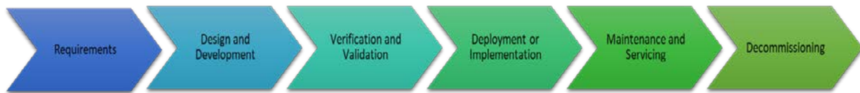
Figure 5: Example of a typical software engineering life cycle approach for product realisation
