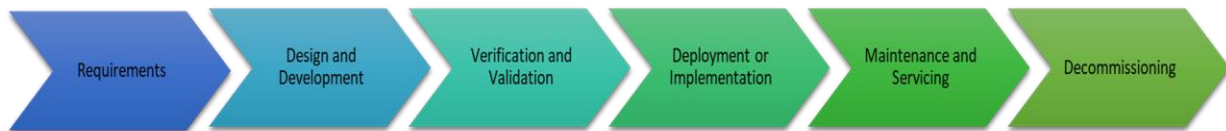
Figure 5: Example of a typical software engineering life cycle approach for product realisation
